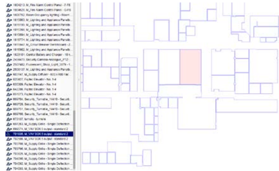
Fig. 10. Georeference of a VAV box in a 2D CAD layout drawing
